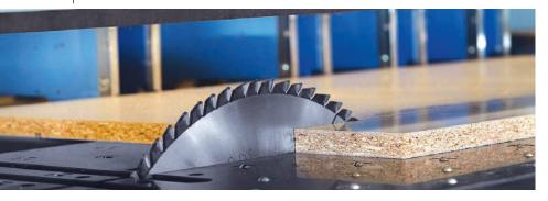
In furniture production, high feed rates and perfect machining results are required for sizing panels, especially when materials and the choice of laminations are constantly changing.
