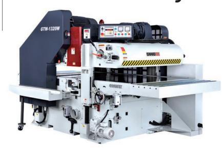
In the field of woodworking, for wider double-side processing, Goodtek Machinery Co provides an alternative to sanding machines – the 1,320-mm GTM-1320W double surface planer.
