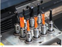
Precision bottom drilling unit Vertical: 9 Bottom vertical drilling bits process bottom side vertical holes on panel
