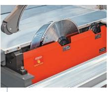
Easy and fast saw-scoring blade changing. Easy scoring adjustment from the front . Entire saw unit on
