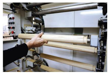
Bacci's T4MO is an innovative CNC turning lathe with four vertical spindles for machining a variety of solid wood elements, including chairs, sofa and table elements, gunstock elements, clothes hangers, knives and hammers handles, musical instruments, sports instruments, etc.
