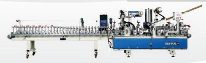
Profile wrapping machine for Door Frames Veneer wrapping UPVC Profile WPC Profile Aluminium Profile
