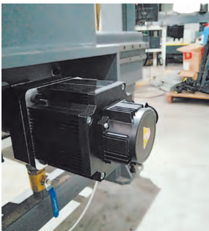
Heavy duty servo motors with Shimpo reducer
