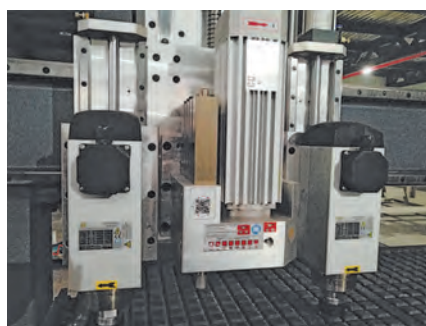
Heavy-duty 2 separate spindles 6 KW with boring head
