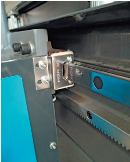
Heavy-duty linear rail & rack & pinion for high cutting speed and accuracy.
