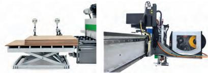
In nesting-based cells, loading and unloading operations are carried out simultaneously, allowing the operator to remove completed components from the unloading station with utmost safety, while the machine is already processing the next panel.
