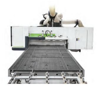
FT Plus allows Biesse clamps to be used to hold solid wood elements or complex small pieces. The extensiveness and increase in payload provide maximum flexibility across machining operations. (Available on sizes 2231 and 2243).
