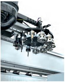
It has electro-spindles for every application – up to 19.2-kW HSD liquid-cooled with automatic tool change HSK F63 1,000-24,000 rpm are available on the machine.
