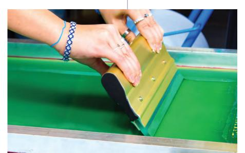
Screen printing is done on long tables, having a length of around 200 feet, which can accommodate more than 20 design papers of 8 feet length. The printing inks are based on starch, which is used as a binder for the pigments.
